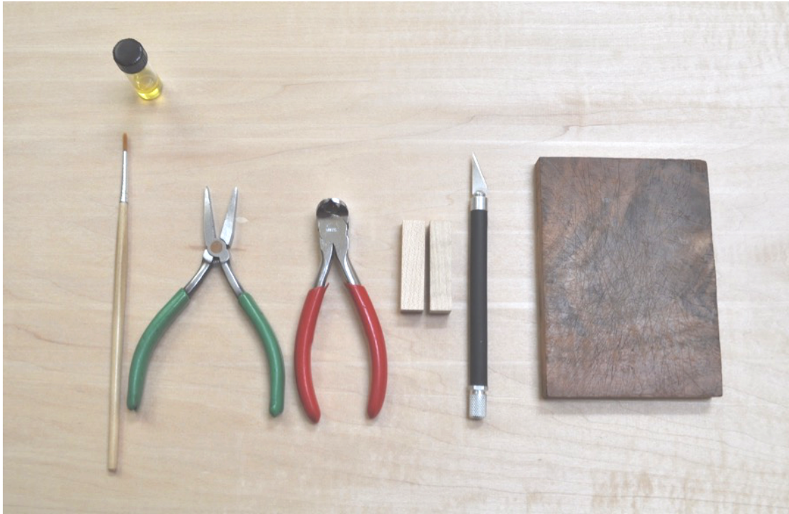
Figure 1. Tools for quill. From left to right; watercolor brush for oil, small jar of oil, smooth-jawed pliers, end nippers, maple voicing blocks, voicing knife, cutting block.
