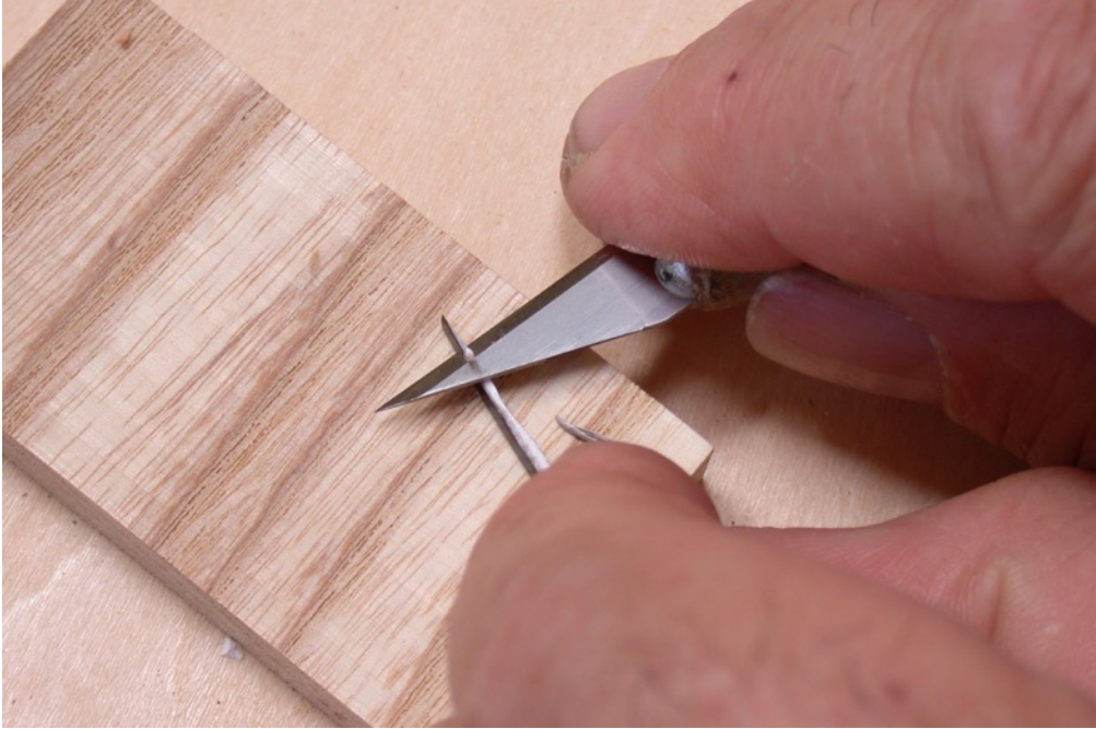
Figure 12. Trimming a side of the end of the shaft.
