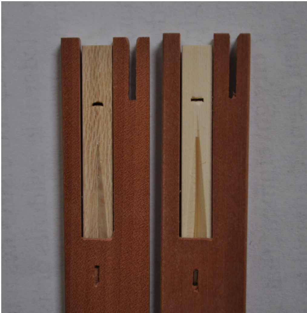
Figure 3. Tongues punched for raven quill (left) and plastic or Canada goose (right). Jacks by Norm Purdy.
